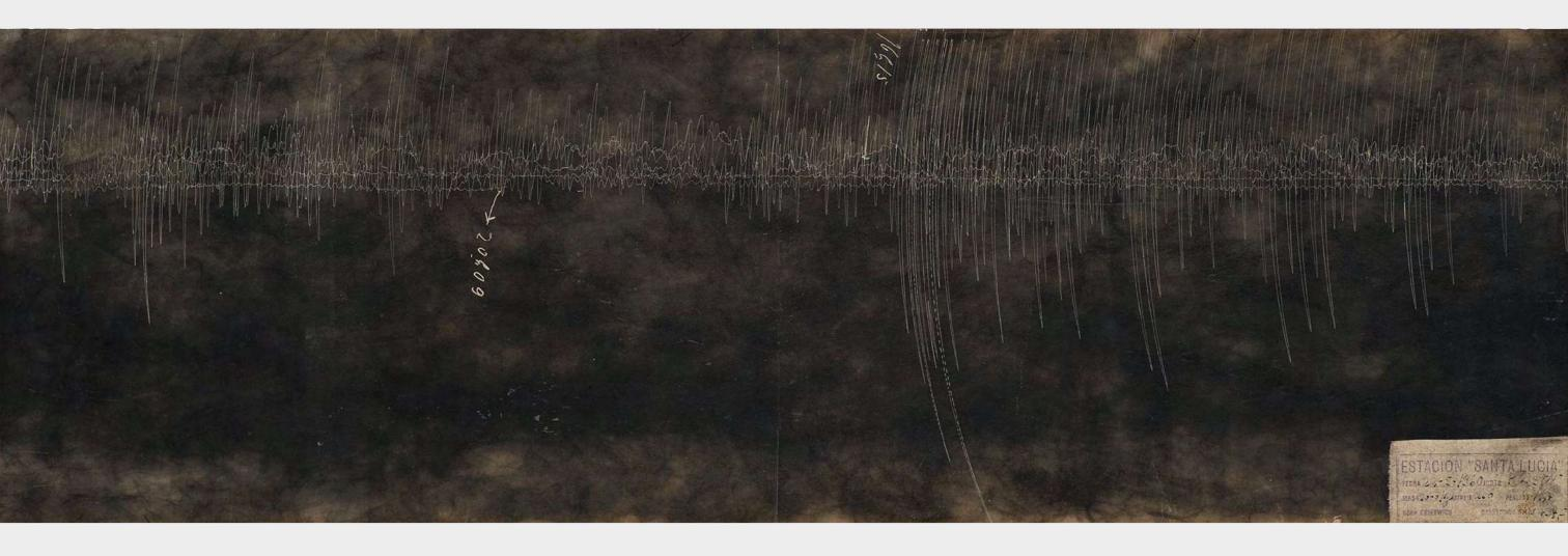
Seismogram corresponding to Fernando Prats' recordings on smoked paper taken at the Cerro Santa Lucía Seismological Station during the largest Earth event ever recorded using an instrument: the 1960 earthquake in southern Chile, the fault-displacement zone which stretched from the Arauco Peninsula to the Taitao Peninsula.
